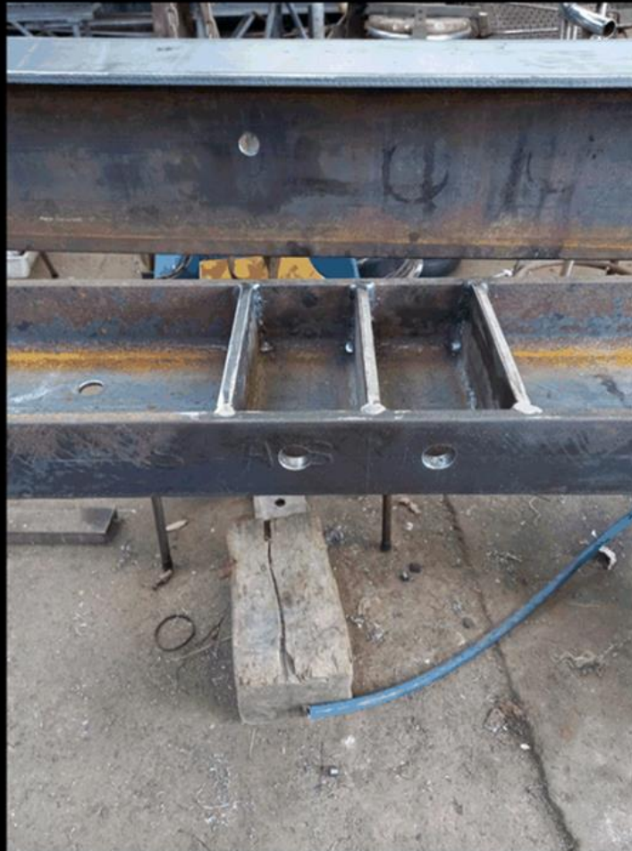
20. WW Pump Station Upgrades - gantry fabrication
